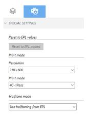
Only resolutions and print modes which are compatible with the color mode of the media profile are available for selection. For example, if the media profile was created for CMYK, only the resolutions and print modes applicable for this color mode are displayed. The Halftone mode should always be set to "Use halftoning from EPL".
